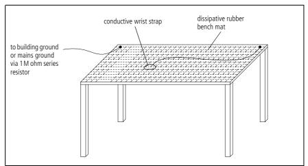
Figure 1.1 Typical Antistatic Bench Set-up
