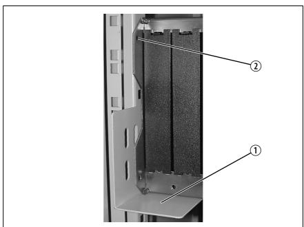
Figure 1.6 Optional Slide Mounting Rail - Rear View
